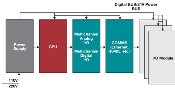
Figure 1: Standard 24V PLC system.
