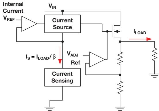
Figure 4: Internal LDO current limit structure.
