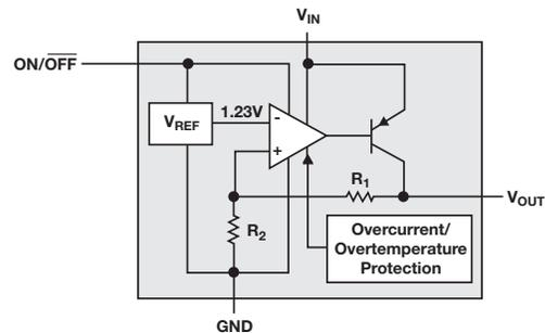
Figure 2: Standard linear regulator.
