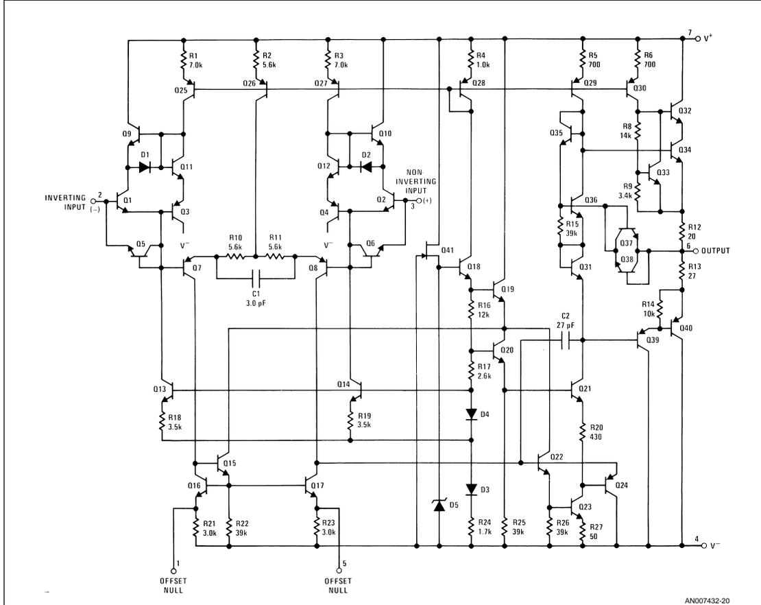
FIGURE 20. Complete Schematic of the LM143
