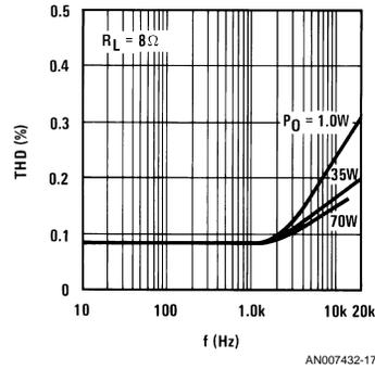
FIGURE 17. Distortion vs Frequency,  $R_L = 8\Omega$
